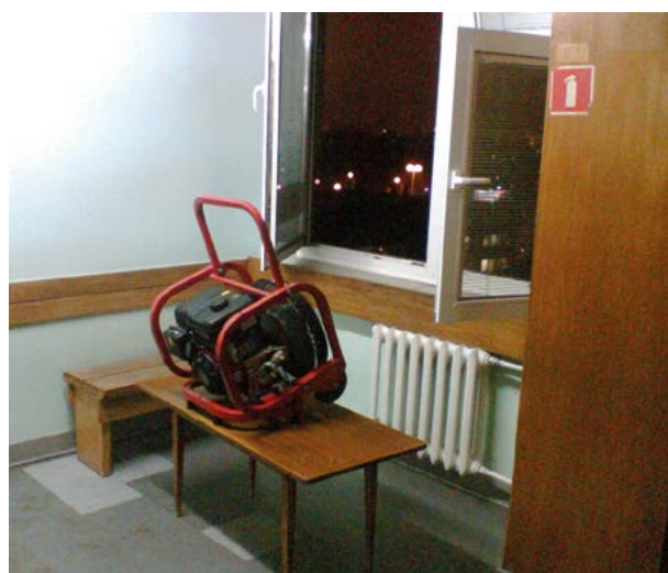
Figure 3. Setting up a fan for negative pressure ventilation
