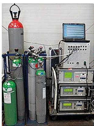
Figure 6. View of the mobile set of SIEMENS analysers used for exhaust gas composition testing
