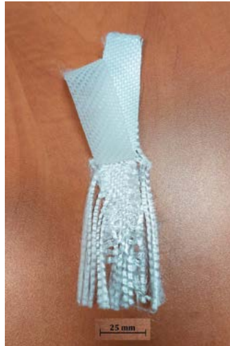
Figure 2. Firefighting hose tape with polyester braid and PVC inner layer
