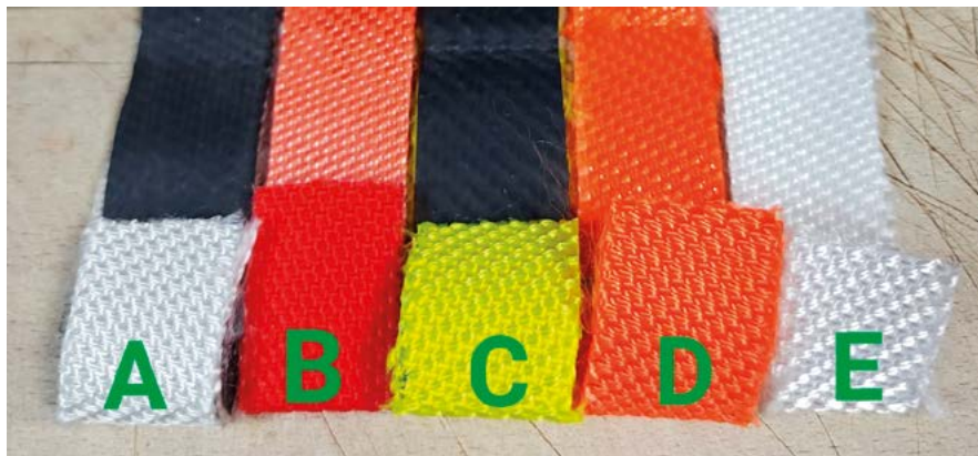
Figure 3. Samples of hose tape (each 25 \pm 0.5 mm wide) showing the variety of polyester braid colours and inner liner types, respectively: A – rubber, B – polyvinyl chloride, C – synthetic EPDM rubber, D – polyurethane, E – polyvinyl chloride
