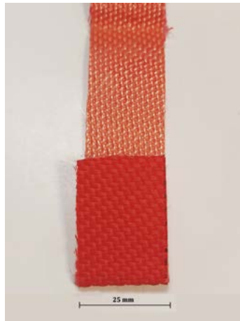
Figure 4. Sample of coated firefighting hose tape, showing styrene-acrylic coated polyester fibre braid and PVC inner lining
