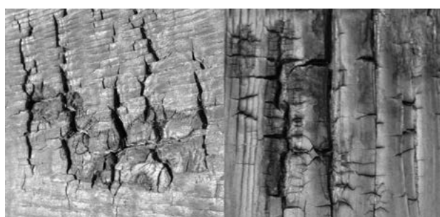
Fig 8. Views of non-treated pine timber specimen after tests with heat source of 10 kW/m 2
