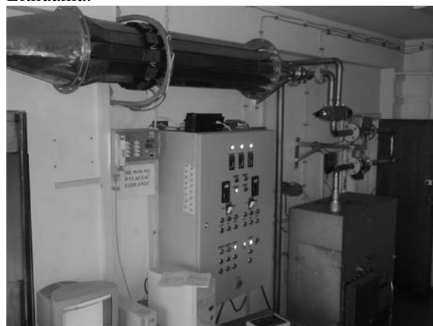
Fig 1. A view of the research equipment for the measurement of the concentration of toxic combustions products
