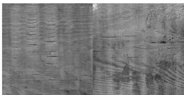
Fig 9. Views of treated pine timber specimen after tests with heat sources of 8 kW/m 2
