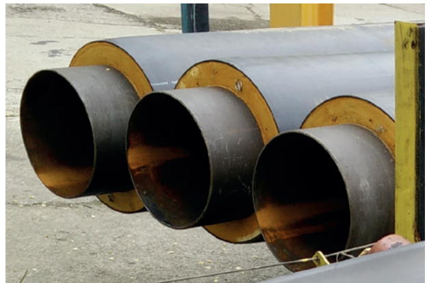
Figure 1b. Manufactured pre-insulated pipes Source: Own elaboration.
