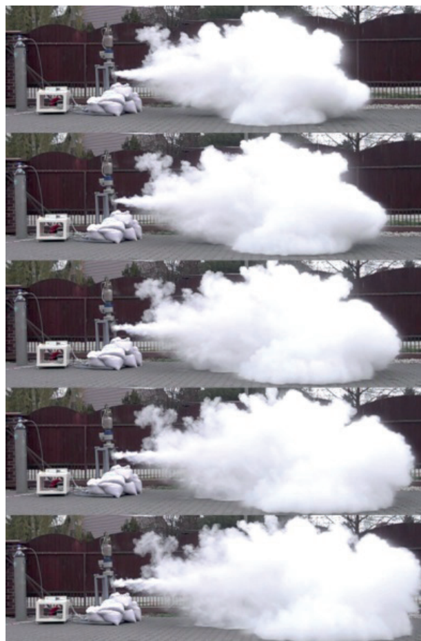
Figure 9. Dispersion of spray powder without nozzle (from above) 60, 70, 80, 90, 100 ms
