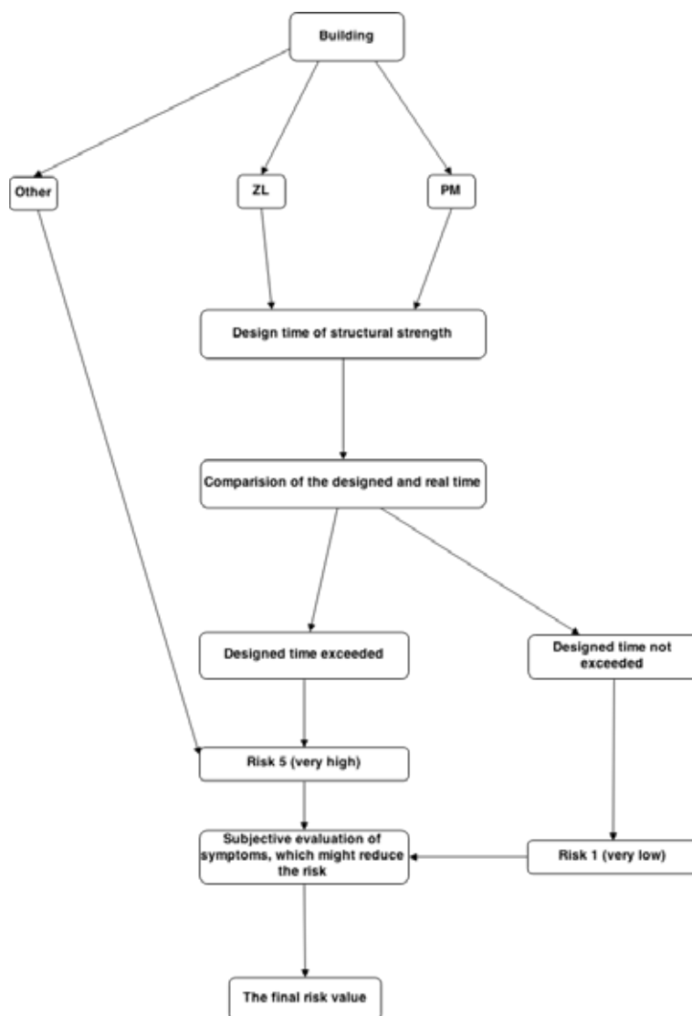
Fig. 1. Activity diagram for modelling of the possible loss of building's load-carrying capacity during a fire Source: Own elaboration.
