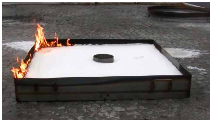
Ryc. 9. Brak całkowitego ugaszenia pożaru testowego wg [19] Fig. 9. Failed to completely extinguish the test fire according to [19]
