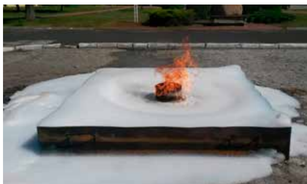
Ryc. 6. Nawrót palenia wg [19] Fig. 6. Burn-back resistance test according to [19]
