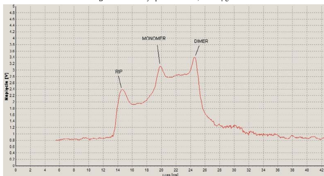
Ryc. 10. Spektrogram reakcji IMS na sarin, c = 380 \mu\text{g}/\text{m}^3 Fig. 10. Ion mobility spectra of sarin, c = 380 \mu\text{g}/\text{m}^3
