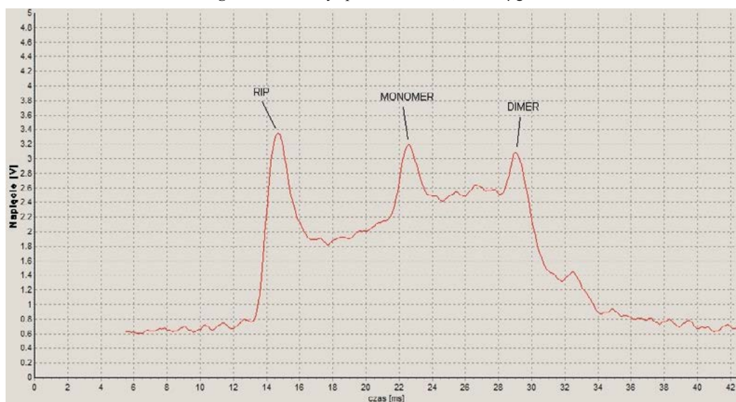
Ryc. 7. Spektrogram reakcji IMS na soman, c = 300 \mu\text{g}/\text{m}^3 Fig. 7. Ion mobility spectra of soman, c = 300 \mu\text{g}/\text{m}^3
