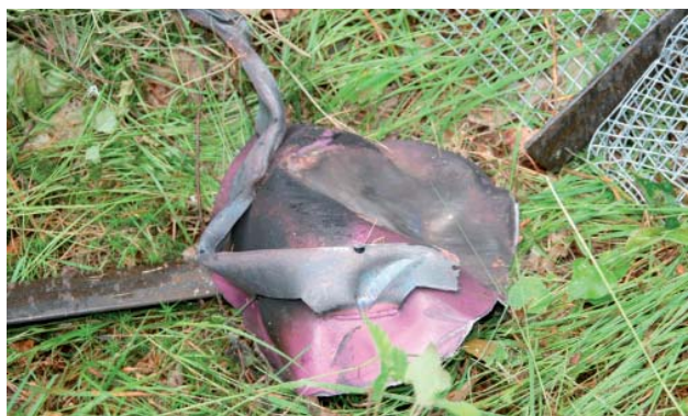
Fig. 7. Down head after explosion.
