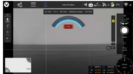
Figure 1. An example of the use of ultrasonic sensors mounted in the Yuneec H520 (marked in red on the left) and the view of the message on the GCS (on the right)
