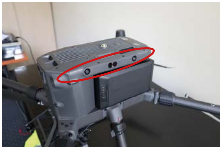
Figure 2. An example of optical sensors mounted in DJI Matrice 300 (on the left) the view of the message on the GCS (on the right)
