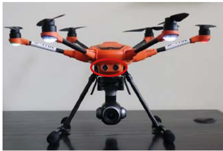
Figure 1. An example of the use of ultrasonic sensors mounted in the Yuneec H520 (marked in red on the left) and the view of the message on the GCS (on the right)
